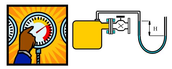
The difference in height between the columns of a manometer is 200 mm with a fluid of density  $900 \text{ kg/m}^3$ . What is the pressure difference? What is the height difference if the same pressure difference is measured using mercury, density  $13600 \text{ kg/m}^3$ , as manometer fluid?
