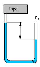
The absolute pressure in a tank is 85 kPa and the local ambient absolute pressure is 97 kPa. If a U-tube with mercury, density 13550 kg/m<sup>3</sup>, is attached to the tank to measure the vacuum, what column height difference would it show?
