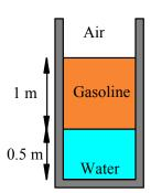
$$\rho_{gasoline} = 750 \text{ kg/m}^3; \quad \rho_{water} = 997 \text{ kg/m}^3$$
