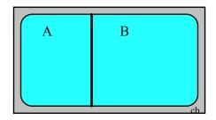
A 1 m<sup>3</sup> container is filled with 400 kg of granite stone, 200 kg dry sand and 0.2 m<sup>3</sup> of liquid 25°C water. Use properties from tables A.3 and A.4. Find the average specific volume and density of the masses when you exclude air mass and volume.
