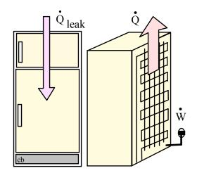
The black grille in the back or at the bottom is the condenser that gives heat to the room air.
