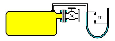
The pressure gauge on an air tank shows 75 kPa when the diver is 10 m down in the ocean. At what depth will the gauge pressure be zero? What does that mean?
