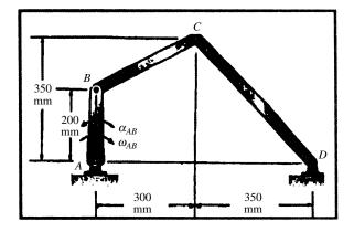
**Problem 17.106** If  $\omega_{AB} = 4$  rad/s counterclockwise and  $\alpha_{AB} = 12$  rad/s<sup>2</sup> counterclockwise, what is the acceleration of point *C*?
