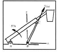
**Problem 17.129** In Problem 17.128, if the angular velocity  $\omega_{AC} = 5^{\circ}$  per second and the angular acceleration  $\alpha_{AC} = -2^{\circ}$  per second squared, determine the angular acceleration of the hydraulic actuator *BC* and the rate of change of the actuator's rate of extension.
