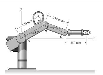
**Solution:** The acceleration of *B* is  $\mathbf{a}_B = \mathbf{a}_A + \boldsymbol{\alpha}_{AB} \times \mathbf{r}_{B/A} - \omega_{AB}^2 \mathbf{r}_{B/A}$ . Evaluating, we get
