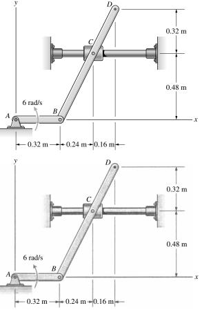
**Problem 17.35** If the crankshaft *AB* rotates at 6000 rpm in the counterclockwise direction, what is the velocity of the piston at the instant shown?
