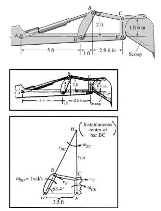
**Solution:** The distance from *D* to *B* is  $r_{BD} = \sqrt{1^2 + 2^2} = 2.24$  ft. The distance from *B* to *H* is
