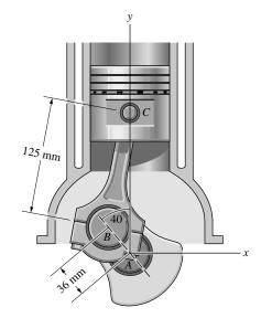
**Solution:** The angle between the crank and the vertical is  $40^\circ$ . The piston is constrained to move in parallel to the *y*-axis. The angular velocity of the crank is:
