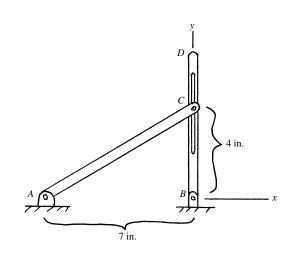
**Problem 17.122** In the system shown in Problem 17.121, the velocity of the pin *C* relative to the slot is 21 in./s upward and is decreasing at 42 in./s<sup>2</sup>. What are the angular velocity and acceleration of bar AC?
