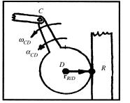
**Problem 17.183** In Problem 17.182, if the rack R of the rack-and-pinion gear is moving upward with a constant velocity of 10 ft/s, what are the angular velocity and acceleration of bar BC?
