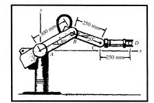
**Problem 17.112** At the instant shown, the dimensions are b = 300 mm, c = 200 mm, d = 150 mm, and e = 260 mm. If link *AB* has a clockwise angular velocity of 0.2 rad/s and a clockwise angular acceleration of 0.06 rad/s<sup>2</sup>, what is the angular acceleration of the excavator's shovel?
