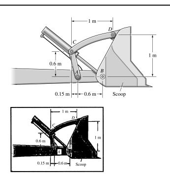
**Problem 17.177** The angular velocity of arm AC in Problem 17.176 is 2 rad/s counterclockwise, and its angular acceleration is 4 rad/s<sup>2</sup> clockwise. What is the angular acceleration of the scoop?
