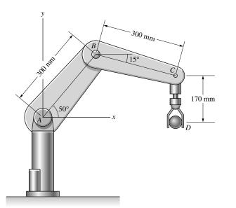
**Solution:** The constraint that the arm *CD* remain vertical means that the angular velocity of arm *CD* is zero. This implies that arm *CD* translates only, and in a translating, non-rotating element the velocity and acceleration at any point is the same, and the velocity and acceleration of arm *CD* is the velocity and acceleration of point *C*. The vectors:
