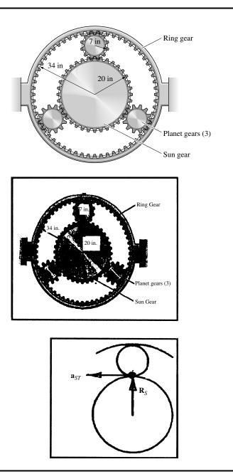
**Problem 17.90** The sun gear in Problem 17.89 has a counterclockwise angular velocity of 4 rad/s and a clockwise angular acceleration of 12 rad/s<sup>2</sup>. What is the magnitude of the acceleration of the centerpoints of the planet gears?
