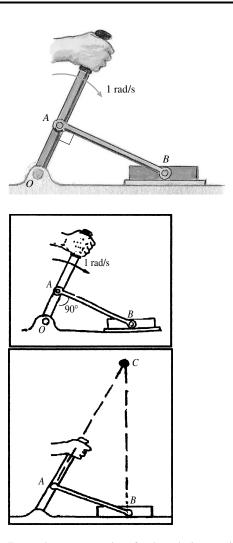
Equate the two expressions for the velocity at point A and separate components,  $5.48i = 27.39\omega_{AB}$ ,  $-2.45j = -12.25\omega_{AB}j$  (one of these conditions is superfluous) and solve to obtain  $\omega_{AB} = 0.2$  rad/s, counterclockwise.
