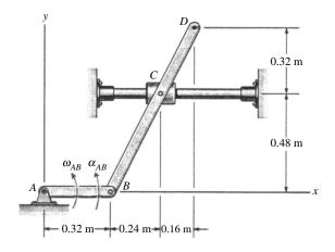
**Problem 17.98** If  $\omega_{AB} = 6$  rad/s and  $\alpha_{AB} = 20$  rad/s<sup>2</sup>, what are the velocity and acceleration of point *C*?
