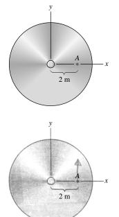
**Problem 17.2** If the angular acceleration of the disk in Problem 17.1 is constant, what are the x and y components of the velocity and acceleration of point A when the disk has rotated  $45^{\circ}$  relative to the position shown?
