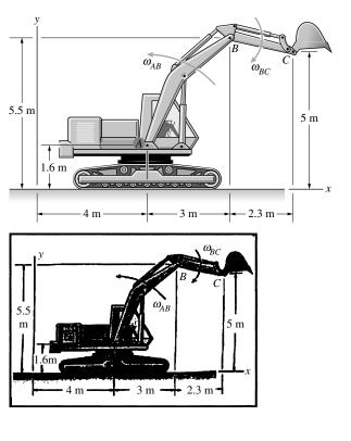
**Problem 17.50** In Problem 17.49, if  $\omega_{AB} = 2$  rad/s, what clockwise angular velocity  $\omega_{BC}$  will cause the vertical component of the velocity of point *C* to be zero? What is the resulting velocity of point *C*?
