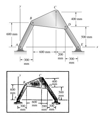
**Solution:** The strategy is analogous to that used in Problem 17.36. The angular velocity of bar *AB* is  $\boldsymbol{\omega} = 4\mathbf{k}$  (rad/s). The radius vector *AB* is  $\mathbf{r}_{B/A} = 300\mathbf{i} + 600\mathbf{j}$  (mm). The velocity of point *B* is
