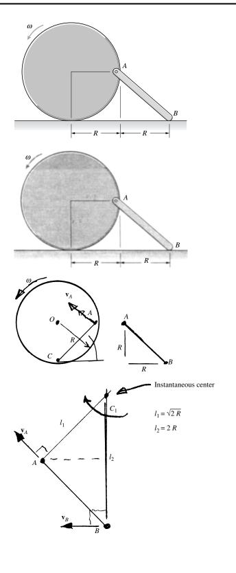
**Problem 17.75** Bar *AB* rotates at 6 rad/s in the clockwise direction. Use instantaneous centers to determine the angular velocity of bar *BC*.
