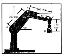
**Problem 17.109** In Problem 17.108, if arm AB has a constant clockwise angular velocity of 0.8 rad/s and you want D to have zero velocity and acceleration, what are the necessary angular velocities and angular accelerations of arms BC and CD?
