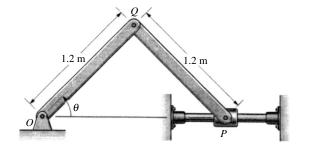
**Problem 17.94** The angle  $\theta = 60^{\circ}$ , and bar *OQ* has a constant counterclockwise angular velocity of 2 rad/s. What is the angular acceleration of the bar *PQ*?
