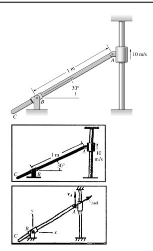
**Problem 17.131** In Problem 17.130, the sleeve at A slides upward at a constant velocity of 10 m/s. Determine the angular acceleration of the bar AC and the rate of change of the velocity at which it slides relative to the sleeve at B.
