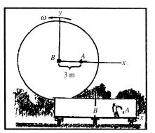
**Problem 17.155** The disk rotates in the horizontal plane about a fixed shaft at the origin with constant angular velocity w = 10 rad/s. The 2-kg slider A moves in a smooth slot in the disk. The spring is unstretched when x = 0 and its constant is k = 400 N/m. Determine the acceleration of A relative to the body-fixed coordinate system when x = 0.4 m.
