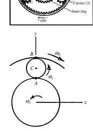
**Problem 17.61** In Problem 17.60, suppose that the outer ring rotates in the clockwise direction at 5 rpm and you want the centerpoints of the carriers to remain stationary during the polishing process. What is the necessary angular velocity of the inner ring?
