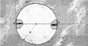
**Problem 17.145** The metal plate is attached to a fixed ball-and-socket support at *O*. The pin *A* slides in a slot in the plate. At the instant shown,  $x_A = 1$  m,  $dx_A/dt = 2$  m/s, and  $d^2x_A/dt^2 = 0$ , and the plate's angular velocity and angular acceleration are  $\omega = 2\mathbf{k}$  (rad/s) and  $\alpha = 0$ . What are the *x*, *y*, and *z* components of the velocity and acceleration of *A* relative to a nonrotating reference frame with its origin at *O*?
