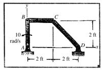
**Problem 17.104** At the instant shown, bar *AB* has no angular velocity but has a counterclockwise angular acceleration of 10 rad/s<sup>2</sup>. Determine the acceleration of point *E*.
