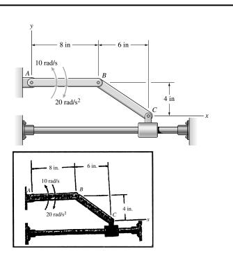
**Problem 17.176** The angular velocity of arm *AC* is 1 rad/s counterclockwise. What is the angular velocity of the scoop?
