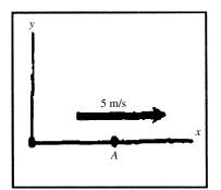
**Problem 17.187** The coordinate system shown is fixed relative to the ship B. The ship uses its radar to measure the position of a stationary buoy A and determines it to be 400i + 200j (m). The ship also measures the velocity of the buoy relative to its body-fixed coordinate system and determines it to be 2i - 8j (m/s). What are the ship's velocity and angular velocity relative to the earth? (Assume that the ship's velocity is in the direction of the y axis).
