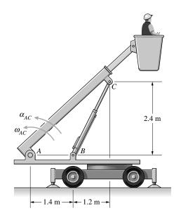
**Solution:** The point C effectively slides in a slot in the arm BC. The angular velocity of
