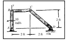
**Problem 17.37** Bar AB rotates at 12 rad/s in the clockwise direction. Determine the angular velocities of bars BC and CD.
