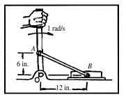
**Problem 17.72** When the mechanism in Problem 17.71 is in the position shown here, use instantaneous centers to determine the horizontal velocity of B.
