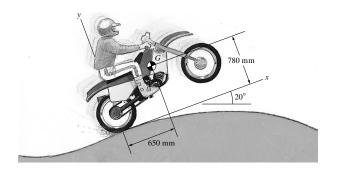
**Solution:** The rear wheel's clockwise angular velocity is  $\omega = (500)(2\pi)/60 = 52.4$  rad/s so the velocity of the center *C* of the wheel is  $\mathbf{v}_C = (52.4)(0.28)\mathbf{i} = 14.7\mathbf{i}$  (m/s). The velocity of the center of mass is
