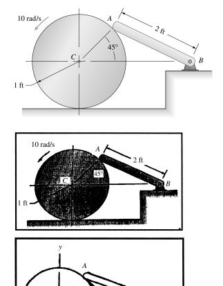
**Solution:** Choose a coordinate system with the origin at the point of contact between the disk and the plane surface, with the x axis parallel to the plane surface. Let A be the point of the bar in contact with the disk. The vector location of point A on the disk is
