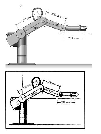
**Problem 17.57** Consider the robot shown in Problem 17.56. Link *AB* is rotating at 2 rad/s in the counterclockwise direction, and link *BC* is rotating at 3 rad/s in the clockwise direction. If you want the velocity of point *D* to be parallel to the *x* axis, what is the necessary angular velocity of link *CD*? What is the resulting velocity of point *D*?
