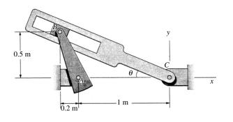
**Problem 17.128** The angular velocity  $\omega_{AC} = 5^{\circ}$  per second. Determine the angular velocity of the hydraulic actuator *BC* and the rate at which the actuator is extending.
