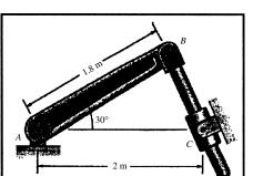
**Problem 17.181** In Problem 17.180, arm *AB* is rotating with an angular velocity of 10 rad/s and an angular acceleration of 20 rad/s<sup>2</sup>, both in the clockwise direction. Determine the angular acceleration of arm *BC*.
