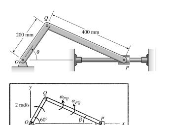
**Solution:** By applying the law of sines, the angle  $\beta = 25.7^{\circ}$ The velocity of Q is  $\mathbf{v}_Q = \mathbf{v}_0 + \boldsymbol{\omega}_{0Q} \times \mathbf{r}_{Q/O}$
