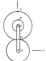
**Problem 17.115** The connecting rod in Problem 17.114 has a counterclockwise angular velocity of 4 rad/s and a clockwise angular acceleration of 12 rad/s<sup>2</sup>. Determine the magnitude of the acceleration at point A.
