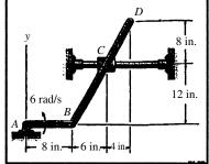
**Problem 17.166** In Problem 17.165, bar AB rotates with a constant angular acceleration of 6 rad/s in the counterclockwise direction. Determine the acceleration of point D.
