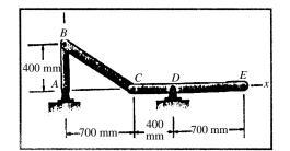
**Problem 17.105** If  $\omega_{AB} = 12$  rad/s and  $\alpha_{AB} = 100$  rad/s<sup>2</sup>, what are the angular accelerations of bars *BC* and *CD*?
