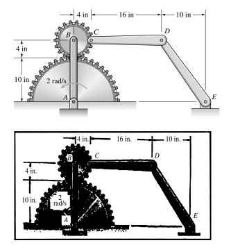
**Problem 17.64** If the bar has a clockwise angular velocity of 10 rad/s and  $v_A = 20$  m/s, what are the coordinates of its instantaneous center of the bar, and what is the value of  $v_B$ ?
