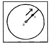
**Problem 17.144** A disk-shaped space station of radius R rotates with constant angular velocity  $\omega$  about the axis perpendicular to the page. Two persons A and B are stationary relative to the station. The coordinate system shown has its origin at B's location and is fixed with respect to the station.
