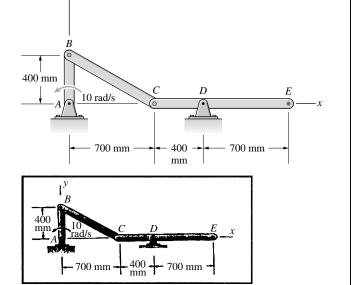
**Problem 17.41** Bar AB rotates at 4 rad/s in the counterclockwise direction. Determine the velocity of point C.
