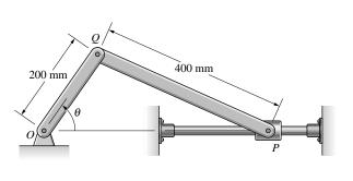
**Solution:** By applying the law of sines,  $\beta = 25.7^{\circ}$ . The velocity of Q is
