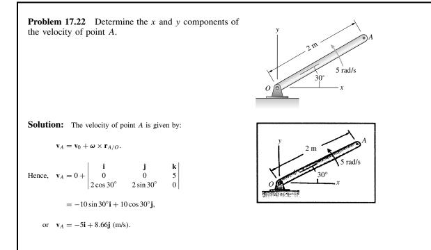
**Problem 17.23** If the angular velocity of the bar in Problem 17.22 is constant, what are the x and y components of the velocity of Point A 0.1 s after the instant shown?
