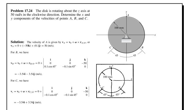
**Problem 17.25** Consider the rotating disk shown in Problem 17.24. If the magnitude of the velocity of point A relative to point B is 4 m/s, what is the magnitude of the disk's angular velocity?
