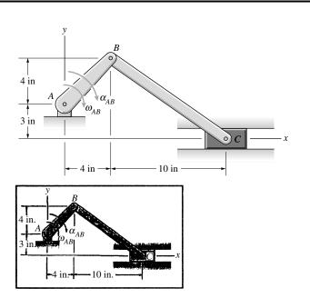
**Problem 17.99** A motor rotates the circular disk mounted at *A*, moving the saw back and forth. (The saw is supported by horizontal slot so that point *C* moves horizontally.) The radius *AB* is 4 in., and the link BC is 14 in. long. In the position shown,  $\theta = 45^{\circ}$  and the link *BC* is horizontal. If the disk has a constant angular velocity of one revolution per second counterclockwise, what is the acceleration of the saw?
