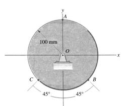
**Problem 17.26** The car is moving to the right at 100 km/hr. The tire is 600 mm in diameter.
