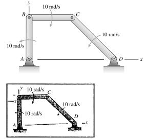
**Solution:** The strategy is to use the definition of angular velocity, including the application of the right hand rule. For bar AB the magnitude is 10 rad/s, and the right hand rule indicates a direction in the positive z direction. (out of the paper).
