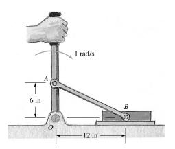
**Solution:** The instantaneous center of OA lies at O, by definition, since O is the point of zero velocity, and the velocity at point A is parallel to the *x*-axis:
