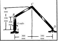
**Problem 17.38** Bar CD rotates at 2 rad/s in the clockwise direction. Determine the angular velocities of bars AB and BC.
