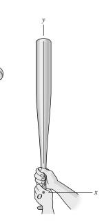
**Solution:** Let  $(x_C, y_C)$  be the coordinates of the instantaneous center. The vector from the instantaneous center to point *O* is  $\mathbf{r}_{O/C} = -x_C \mathbf{i} - y_C \mathbf{j}$  (ft). The velocity of point *O* is
