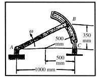
**Problem 17.137** Suppose that the curved bar in Example 17.9 has a clockwise angular velocity of 4 rad/s and a counterclockwise angular acceleration of 10 rad/s<sup>2</sup>. What is the angular acceleration of bar AB?
