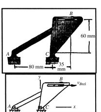
**Problem 17.125** In the system shown in Problem 17.124, the bar *AB* has an angular velocity of 4 rad/s in the clockwise direction and an angular acceleration of 10 rad/s<sup>2</sup> in the counterclockwise direction. What is the acceleration of pin *B* relative to the slot?
