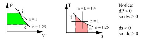
Notice this process has some heat transfer in during expansion which is unusual. The typical process would have n = 1.5 with a heat loss.
