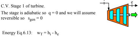
Entropy Eq.9.8:  $s_e = s_i + \int dq/T + s_{gen} = s_i + 0 + 0$ Inlet state: B.1.3:  $h_i = 4114.9 \text{ kJ/kg}$ ,  $s_i = 7.4077 \text{ kJ/kg K}$ Exit state: 800 kPa,  $s = s_i$
