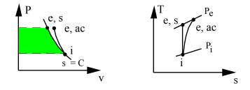
Assume an actual compressor has the same exit pressure and specific heat transfer as the ideal isothermal compressor in Problem 9.8 with an isothermal efficiency of 80%. Find the specific work and exit temperature for the actual compressor.
