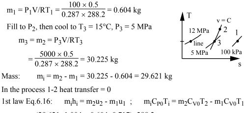
$$T_2 = \frac{(29.621 \times 1.004 + 0.604 \times 0.717) \times 288.2}{30.225 \times 0.717} = 401.2 \text{ K}$$
