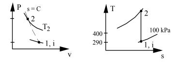
Air in a tank is at 300 kPa, 400 K with a volume of 2  $m^3$ . A valve on the tank is opened to let some air escape to the ambient to a final pressure inside of 200 kPa. At the same time the tank is heated so the air remaining has a constant temperature. What is the mass average value of the s leaving assuming this is an internally reversible process?
