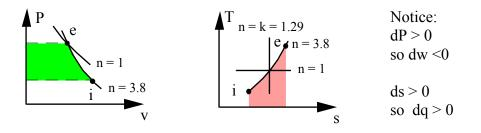
Notice process is externally irreversible,  $\Delta T$  between source and  $CO_2$
