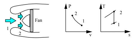
A compressor receives air at 290 K, 100 kPa and a shaft work of 5.5 kW from a gasoline engine. It should deliver a mass flow rate of 0.01 kg/s air to a pipeline. Find the maximum possible exit pressure of the compressor.
