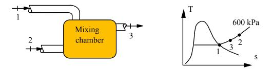
The mixing process generates entropy. The two inlet flows could have exchanged energy (they have different T) through some heat engines and produced work, the process failed to do that, thus irreversible.
