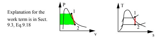
Inlet state: Table B.1.3  $h_i = 3344 \text{ kJ/kg}, s_i = 7.0833 \text{ kJ/kg K}$
