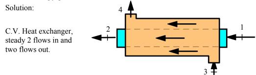
Energy Eq.6.10:  $\dot{m}_{O2}h_1 + \dot{m}_{N2}h_3 = \dot{m}_{O2}h_2 + \dot{m}_{N2}h_4$ Same exit temperature so  $T_4 = T_2$  with values from Table A.5
