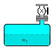
An empty cannister of  $0.002 \text{ m}^3$  is filled with R-134a from a line flowing saturated liquid R-134a at 0°C. The filling is done quickly so it is adiabatic. Find the final mass in the cannister and the total entropy generation.
