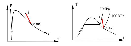
The throttle process described in Example 6.5 is an irreversible process. Find the entropy generation per kg ammonia in the throttling process.
