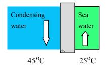
$$\frac{\mathrm{dS}}{\mathrm{dt}} = 0 = \sum \frac{\dot{Q}}{T} + \dot{S}_{gen} = \frac{\dot{Q}}{T_{45}} - \frac{\dot{Q}}{T_{25}} + \dot{S}_{gen}$$
