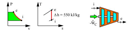
A compressor is surrounded by cold R-134a so it works as an isothermal compressor. The inlet state is 0°C, 100 kPa and the exit state is saturated vapor. Find the specific heat transfer and specific work.
