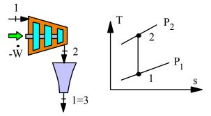
Separate control volumes around compressor and nozzle. For ideal compressor we have inlet : 1 and exit : 2
