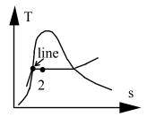
An old abandoned saltmine,  $100\ 000\ m^3$  in volume, contains air at 290 K, 100 kPa. The mine is used for energy storage so the local power plant pumps it up to 2.1 MPa using outside air at 290 K, 100 kPa. Assume the pump is ideal and the process is adiabatic. Find the final mass and temperature of the air and the required pump work.
