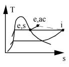
A water-cooled air compressor takes air in at 20°C, 90 kPa and compresses it to 500 kPa. The isothermal efficiency is 80% and the actual compressor has the same heat transfer as the ideal one. Find the specific compressor work and the exit temperature.
