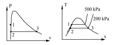
Two flowstreams of water, one at 0.6 MPa, saturated vapor, and the other at 0.6 MPa, 600°C, mix adiabatically in a steady flow process to produce a single flow out at 0.6 MPa, 400°C. Find the total entropy generation for this process. Solution:
