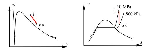
Steam enters a turbine at 3 MPa, 450°C, expands in a reversible adiabatic process and exhausts at 10 kPa. Changes in kinetic and potential energies between the inlet and the exit of the turbine are small. The power output of the turbine is 800 kW. What is the mass flow rate of steam through the turbine?
