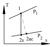
The small turbine in Problem 9.38 was ideal. Assume instead the isentropic turbine efficiency is 88%. Find the actual specific turbine work and the entropy generated in the turbine.
