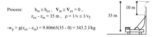
The velocity in nozzle is such that it can rise 10 m, so make that column C.V.
