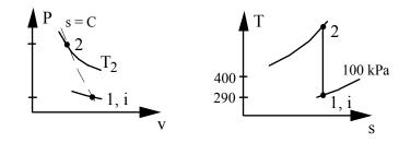
Calculate the air temperature and pressure at the stagnation point right in front of a meteorite entering the atmosphere (-50 °C, 50 kPa) with a velocity of 2000 m/s. Do this assuming air is incompressible at the given state and repeat for air being a compressible substance going through an adiabatic compression.
