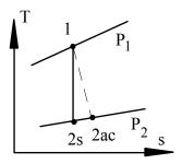
A turbine receives air at 1500 K, 1000 kPa and expands it to 100 kPa. The turbine has an isentropic efficiency of 85%. Find the actual turbine exit air temperature and the specific entropy increase in the actual turbine.
