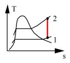
A boiler section boils 3 kg/s saturated liquid water at 2000 kPa to saturated vapor in a reversible constant pressure process. Assume you do not know that there is no work. Prove that there is no shaftwork using the first and second laws of thermodynamics.
