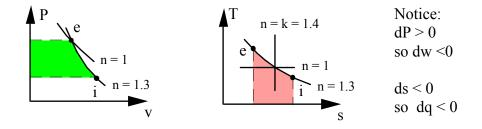
A flow of 4 kg/s ammonia goes through a device in a polytropic process with an inlet state of 150 kPa, -20°C and an exit state of 400 kPa, 80°C. Find the polytropic exponent n, the specific work and heat transfer.
