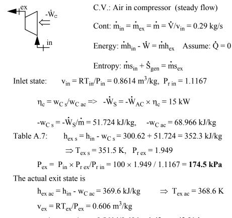
$$\label{eq:rho_ex} \begin{split} \rho_{ex}/\rho_{in} &= v_{in}/v_{ex} = 0.8614/0.606 = \textbf{1.42} \ \text{ or } \ \textbf{42 \% increase} \\ s_{gen} &= s_{ex} - s_{in} = 7.0767 - 6.8693 - 0.287 \ln(174/100)] = \textbf{0.0484 kJ/kg K} \end{split}$$
