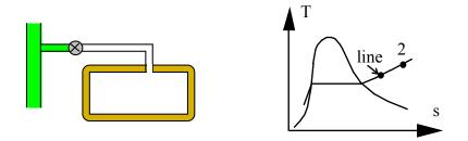
Air from a line at 12 MPa, 15°C, flows into a 500-L rigid tank that initially contained air at ambient conditions, 100 kPa, 15°C. The process occurs rapidly and is essentially adiabatic. The valve is closed when the pressure inside reaches some value,  $P_2$ . The tank eventually cools to room temperature, at which time the pressure inside is 5 MPa. What is the pressure  $P_2$ ? What is the net entropy change for the overall process?
