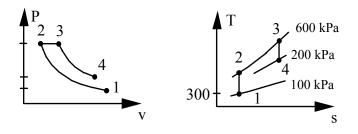
A certain industrial process requires a steady 0.5 kg/s supply of compressed air at 500 kPa, at a maximum temperature of 30°C. This air is to be supplied by installing a compressor and aftercooler. Local ambient conditions are 100 kPa, 20°C. Using an reversible compressor, determine the power required to drive the compressor and the rate of heat rejection in the aftercooler. Solution:
