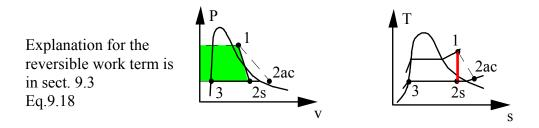
$$w_{T,AC} = \eta \times w_{T,s} = 1229.9 \text{ kJ/kg}$$
