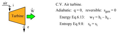
a) Table A.7:  $h_i = 1277.8 \text{ kJ/kg}, s_{Ti}^0 = 8.34596 \text{ kJ/kg K}$
