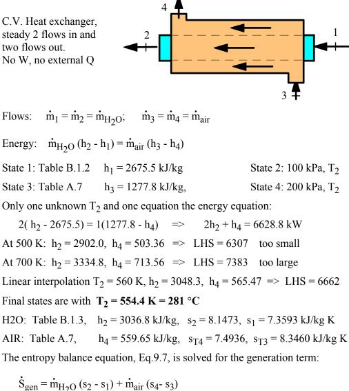
= 2(8.1473 - 7.3593) + 1 (7.4936 - 8.3460) = 0.724 kW/KNo pressure correction is needed as the air pressure for 4 and 3 is the same.
