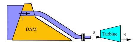
States: compressed liquid B.1.1  $v_2 \approx v_1 \approx v_f = 0.001002 \text{ m}^3/\text{kg}$
