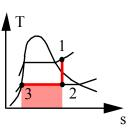
One technique for operating a steam turbine in part-load power output is to throttle the steam to a lower pressure before it enters the turbine, as shown in Fig. P9.39. The steamline conditions are 2 MPa, 400°C, and the turbine exhaust pressure is fixed at 10 kPa. Assuming the expansion inside the turbine to be reversible and adiabatic, determine
