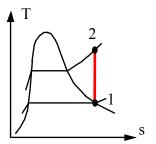
In a heat pump that uses R-134a as the working fluid, the R-134a enters the compressor at 150 kPa,  $-10^{\circ}$ C at a rate of 0.1 kg/s. In the compressor the R-134a is compressed in an adiabatic process to 1 MPa. Calculate the power input required to the compressor, assuming the process to be reversible.
