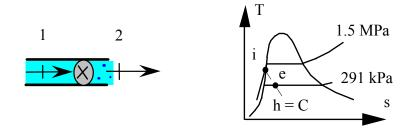
A geothermal supply of hot water at 500 kPa, 150°C is fed to an insulated flash evaporator at the rate of 1.5 kg/s. A stream of saturated liquid at 200 kPa is drained from the bottom of the chamber and a stream of saturated vapor at 200 kPa is drawn from the top and fed to a turbine. Find the rate of entropy generation in the flash evaporator.
