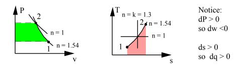
Carbon dioxide flows through a device entering at 300 K, 200 kPa and leaving at 500 K. The process is steady state polytropic with n = 3.8 and heat transfer comes from a 600 K source. Find the specific work, specific heat transfer and the specific entropy generation due to this process.
