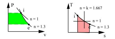
Air at 100 kPa, 300 K, flows through a device at steady state with the exit at 1000 K during which it went through a polytropic process with n = 1.3. Find the exit pressure, the specific work and heat transfer.
