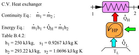
Notice we can find  $\dot{Q}_{H}$  but the temperature  $T_{H}$  is not constant making it difficult to evaluate the COP of the heat pump.
