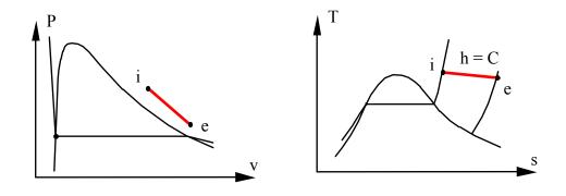
Remark: Since process is irreversible there is no area under curve in T-s diagram that correspond to a q, nor is there any area in the P-v diagram corresponding to a shaft work.
