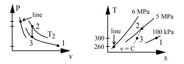
Problem could have been solved with constant specific heats from A.5 in which case we would get the energy explicit in  $T_2$  (no iterations).
