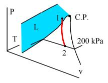
A piston/cylinder arrangement contains water of quality x = 0.7 in the initial volume of  $0.1 \text{ m}^3$ , where the piston applies a constant pressure of 200 kPa. The system is now heated to a final temperature of 200°C. Determine the work and the heat transfer in the process.
