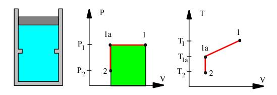
A spring loaded piston/cylinder contains 1.5 kg of air at 27C and 160 kPa. It is now heated to 900 K in a process where the pressure is linear in volume to a final volume of twice the initial volume. Plot the process in a P-v diagram and find the work and heat transfer.
