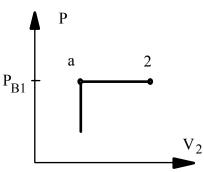
A small flexible bag contains 0.1 kg ammonia at  $-10^{\circ}$ C and 300 kPa. The bag material is such that the pressure inside varies linear with volume. The bag is left in the sun with with an incident radiation of 75 W, loosing energy with an average 25 W to the ambient ground and air. After a while the bag is heated to  $30^{\circ}$ C at which time the pressure is 1000 kPa. Find the work and heat transfer in the process and the elapsed time.
