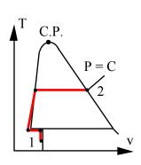
Water is in a piston cylinder maintaining constant P at 700 kPa, quality 90% with a volume of 0.1 m<sup>3</sup>. A heater is turned on heating the water with 2.5 kW. What is the rate of mass (kg/s) vaporizing?
