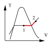
A 1-L capsule of water at 700 kPa, 150°C is placed in a larger insulated and otherwise evacuated vessel. The capsule breaks and its contents fill the entire volume. If the final pressure should not exceed 125 kPa, what should the vessel volume be?
