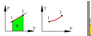
Air in a piston/cylinder at 200 kPa, 600 K, is expanded in a constant-pressure process to twice the initial volume (state 2), shown in Fig. P5.101. The piston is then locked with a pin and heat is transferred to a final temperature of 600 K. Find *P*, *T*, and *h* for states 2 and 3, and find the work and heat transfer in both processes.
