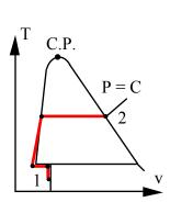
A piston/cylinder assembly contains 1 kg of liquid water at  $20^{\circ}$ C and 300 kPa. There is a linear spring mounted on the piston such that when the water is heated the pressure reaches 1 MPa with a volume of  $0.1 \text{ m}^3$ . Find the final temperature and the heat transfer in the process.
