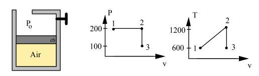
A vertical piston/cylinder has a linear spring mounted as shown so at zero cylinder volume a balancing pressure inside is zero. The cylinder contains 0.25 kg air at 500 kPa, 27°C. Heat is now added so the volume doubles.
