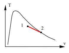
A water-filled reactor with volume of 1 m<sup>3</sup> is at 20 MPa, 360°C and placed inside a containment room as shown in Fig. P5.48. The room is well insulated and initially evacuated. Due to a failure, the reactor ruptures and the water fills the containment room. Find the minimum room volume so the final pressure does not exceed 200 kPa. Solution:
