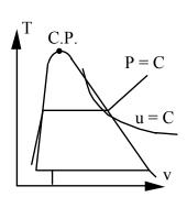
Notice the constant u(h) line becomes parallel to the constant T lines in the superheated vapor region for low P where it is an ideal gas. In the T-v diagram the constant u (h) line becomes horizontal.
