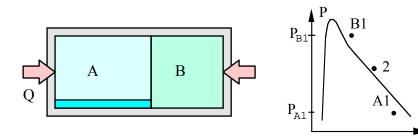
The cylinder volume below the constant loaded piston has two compartments A and B filled with water. A has 0.5 kg at 200 kPa, 150°C and B has 400 kPa with a quality of 50% and a volume of 0.1 m<sup>3</sup>. The valve is opened and heat is transferred so the water comes to a uniform state with a total volume of 1.006 m<sup>3</sup>.
