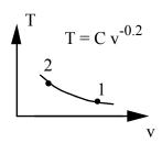
A piston/cylinder contains  $0.001 \text{ m}^3$  air at 300 K, 150 kPa. The air is now compressed in a process in which  $PV^{1.25} = C$  to a final pressure of 600 kPa. Find the work performed by the air and the heat transfer.
