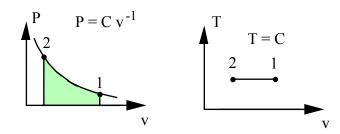
Oxygen at 300 kPa, 100°C is in a piston/cylinder arrangement with a volume of 0.1 m<sup>3</sup>. It is now compressed in a polytropic process with exponent, n = 1.2, to a final temperature of 200°C. Calculate the heat transfer for the process.
