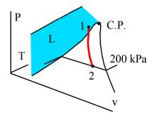
Superheated refrigerant R-134a at 20°C, 0.5 MPa is cooled in a piston/cylinder arrangement at constant temperature to a final two-phase state with quality of 50%. The refrigerant mass is 5 kg, and during this process 500 kJ of heat is removed. Find the initial and final volumes and the necessary work.
