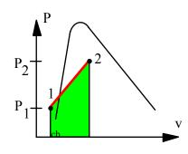
A closed steel bottle contains ammonia at  $-20^{\circ}$ C, x = 20% and the volume is 0.05 m<sup>3</sup>. It has a safety valve that opens at a pressure of 1.4 MPa. By accident, the bottle is heated until the safety valve opens. Find the temperature and heat transfer when the valve first opens.
