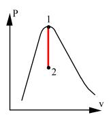
A 10-L rigid tank contains R-22 at  $-10^{\circ}$ C, 80% quality. A 10-A electric current (from a 6-V battery) is passed through a resistor inside the tank for 10 min, after which the R-22 temperature is 40°C. What was the heat transfer to or from the tank during this process?
